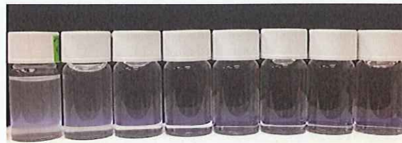
Figure 9. The 8 different concentration calibration solutions of St-DVB copolymer microbeads: From left to right, the concentrations are 100, 50, 20, 10, 5, 2, 1, and 0 mg/L.
