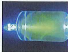
Fig. 2 Fluorescent image of uranine ( C_{20}H_{10}Na_2O_3 ), which is used for the reference material of chlorophyll sensor.
