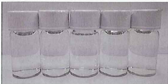
Fig. 3 Uranine samples with different concentrations, which are not distinguishable each other by naked eyes.
